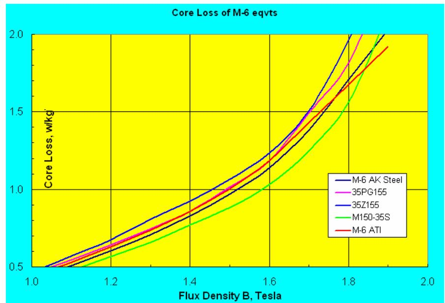
**Fig. 7. Different M-6 Grade steels are optimal at different flux densities.**
