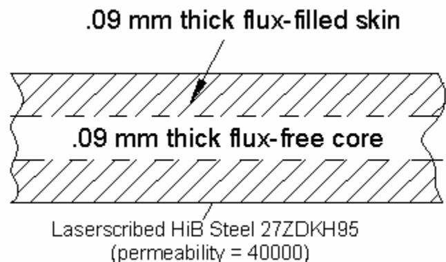
**Fig. 6. Too high permeability can prevent flux from flowing in a central core of a lamination**
