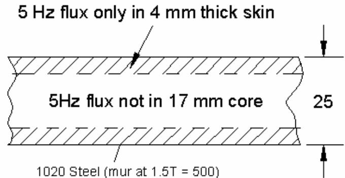
**Fig. 16. The central core of solid steels may not carry AC flux**
