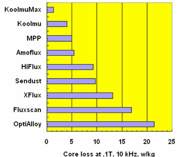
**Fig. 22. Core loss of various alloy powders**
