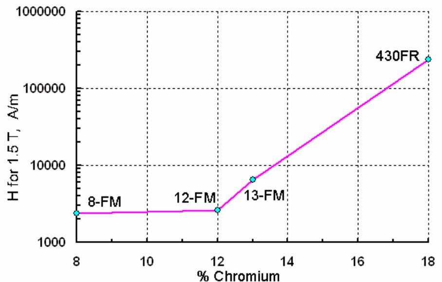
**Fig. 12. Magnetizing current needed depends on grade of stainless steel.**
