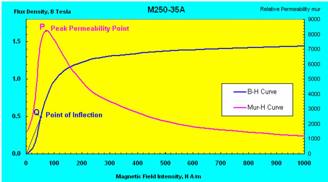
**Fig. 2. B-H Curve has an inflection point. It causes poor convergence**
