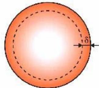
**Fig. 15. AC Flux can be carried only upto the Skin Depth  $\delta$**
