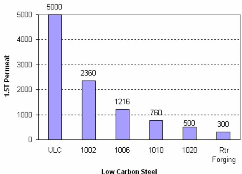
**Fig. 14. Permeability of Low Carbon Steel reduces as %C increases.**
