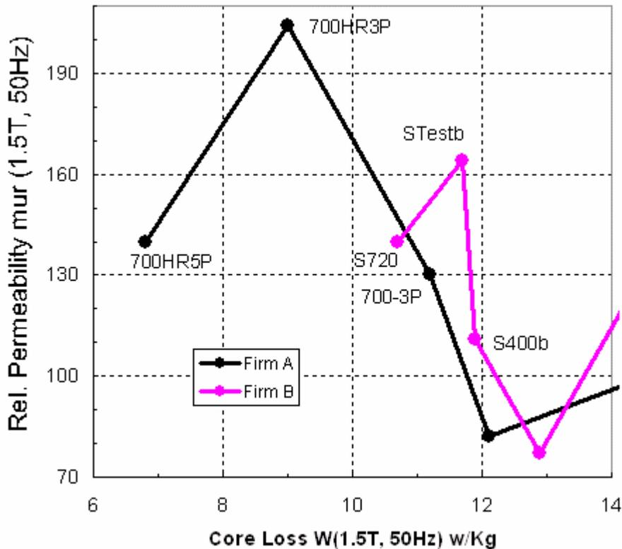
**Fig. 19. Magnetic Property Map of SMC at 1.5T, 50 Hz. Firm A offers superior SMC.**
