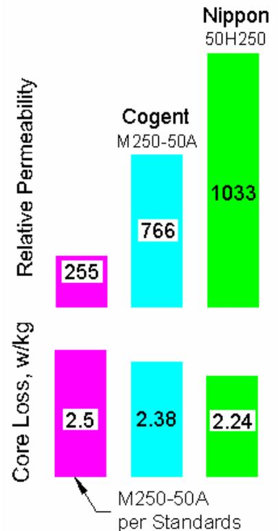
**Fig. 4. Properties of actual steels greatly differ from grade standards.**
