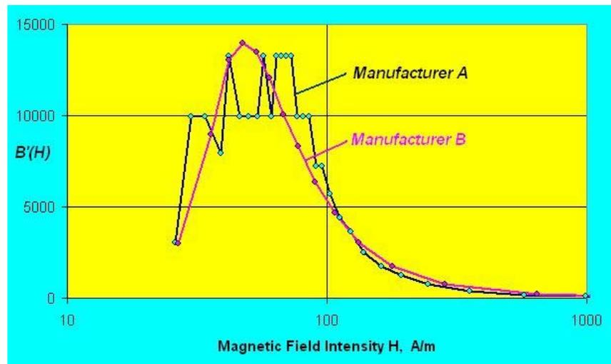
**Fig. 3.  $B'(H)$  curve for firm A's steel has digitization noise.**
