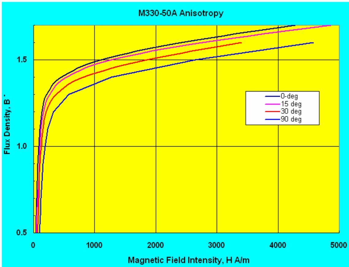
**Fig. 5. Magnetic Properties of NGO steels vary somewhat with direction.**
