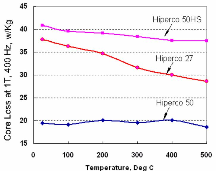
**Fig. 11. Hiperco 27's Core Loss beneficially decreases with temperature,**
