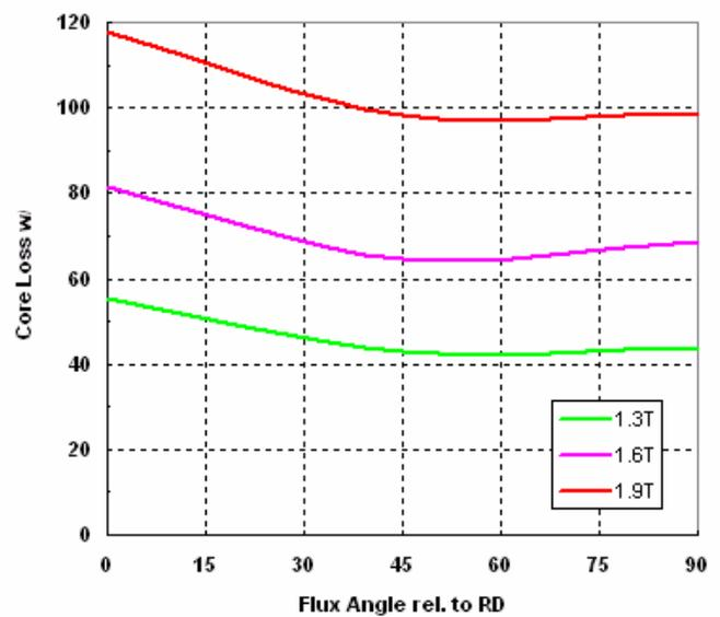
**Fig. 10. Core Loss of Cobalt Steels varies with direction of flux.**
