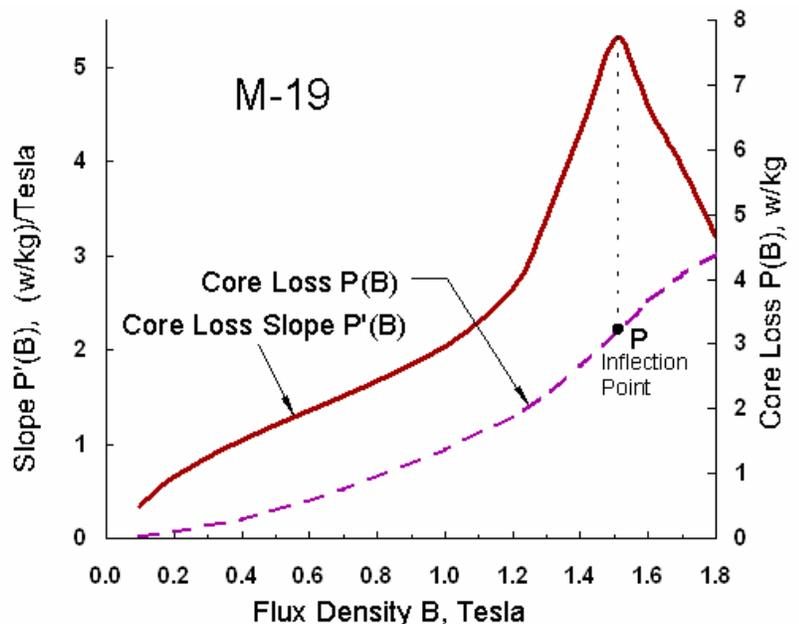
**Fig. 8. Core Loss Curve also have an Inflection Point P.**
