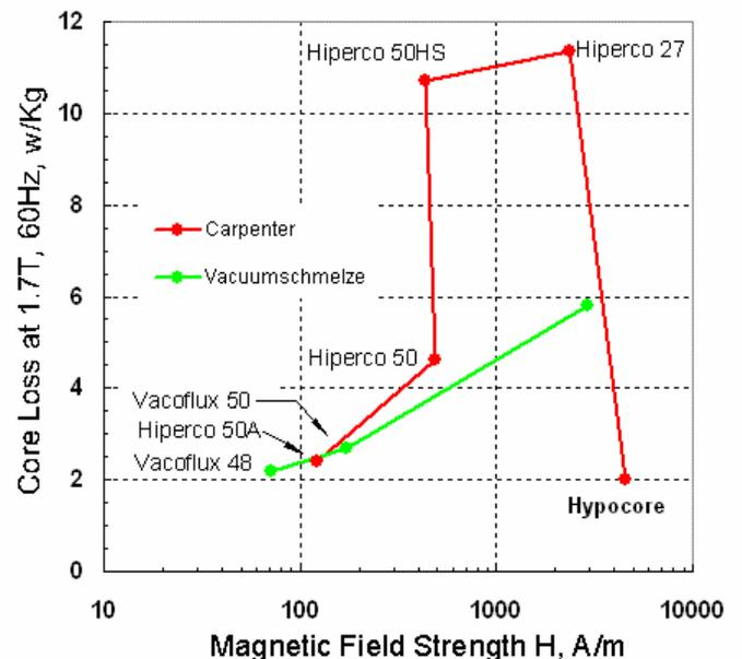
**Fig. 9. Vacoflux 48 produces least core loss and copper loss. But Hypocore incurs more copper loss (it needs more magnetizing current to reach same B.)**
